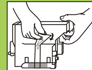
6. Install the new toner kit into the printer, make sure the color of the toner kit matches the corresponding toner kit slot on the printer, then guide the cartridge until it snaps into place.
