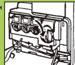
3. Hold the used toner kit and pull it out from the printer.
